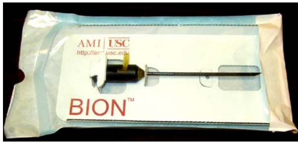
FIGURE 2. The BIT loaded with a BION, in sterile packaging ready for shipping. Note the window cut-out in the cardboard tray beneath the BION chamber, to allow functional testing after packaging and sterilization.
